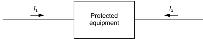
Figure 3. Definition of the current phasors at both sides of the protected equipment respecting Kirchhoff's current law.
